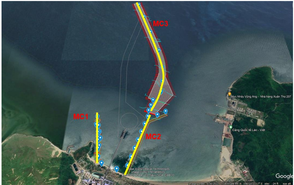
Figure 2.15. Schematic of cross-section lines evaluating the physical characteristics of dredged material
